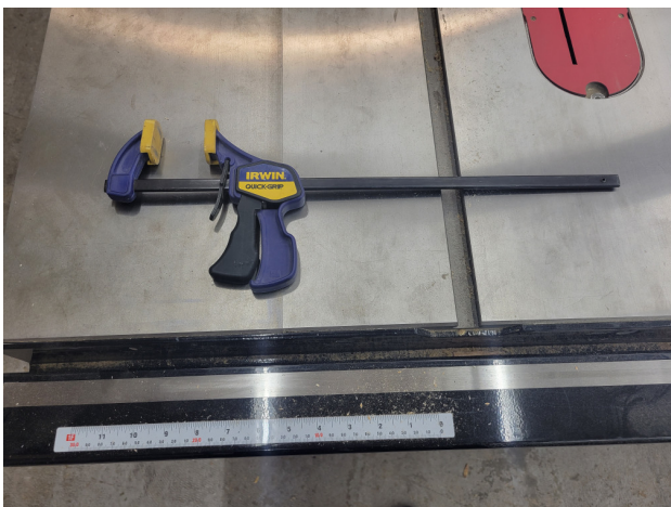
Highly Recommended: Clamps to hold rails and spacers in place when no factory holes are present.
