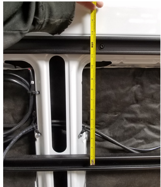
Reference: The upper rail hole line is about 1' above the lower rail hole line.
