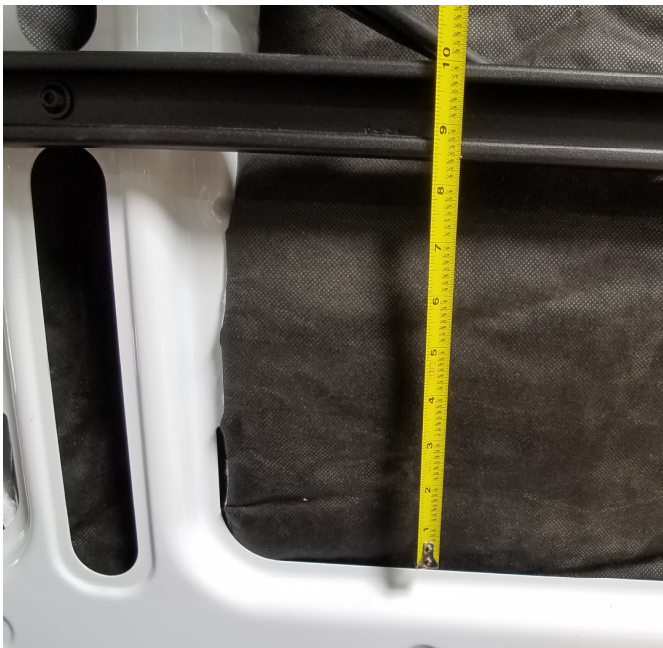
Reference: The lower rail hole line is about 9.5" above the bottom of the cutouts near the bottom of the van.
