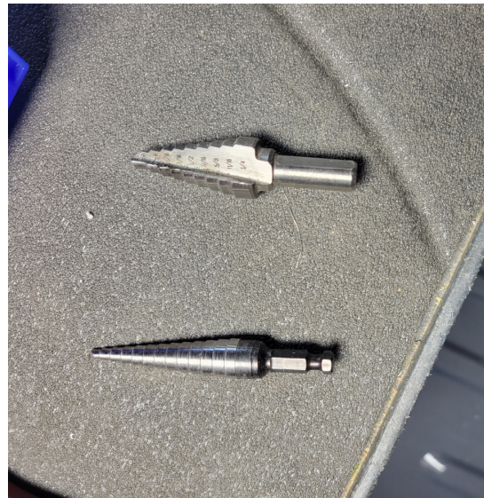
Required: 11/16" step bit (top). The bottom narrower bit is helpful getting the widening started, but is not required. The 11/16" bit (top) is the only one required for the install.
