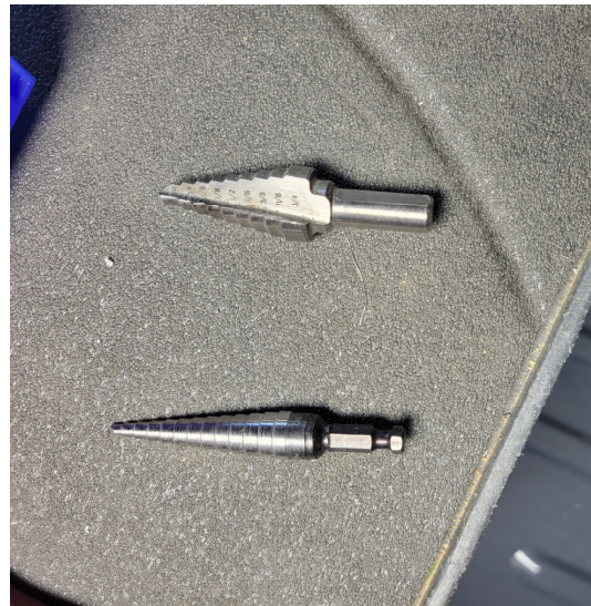
Required: 11/16" step bit (top). The bottom narrower bit is helpful getting the widening started, but is not required. The 11/16" bit (top) is the only one required for the install.
