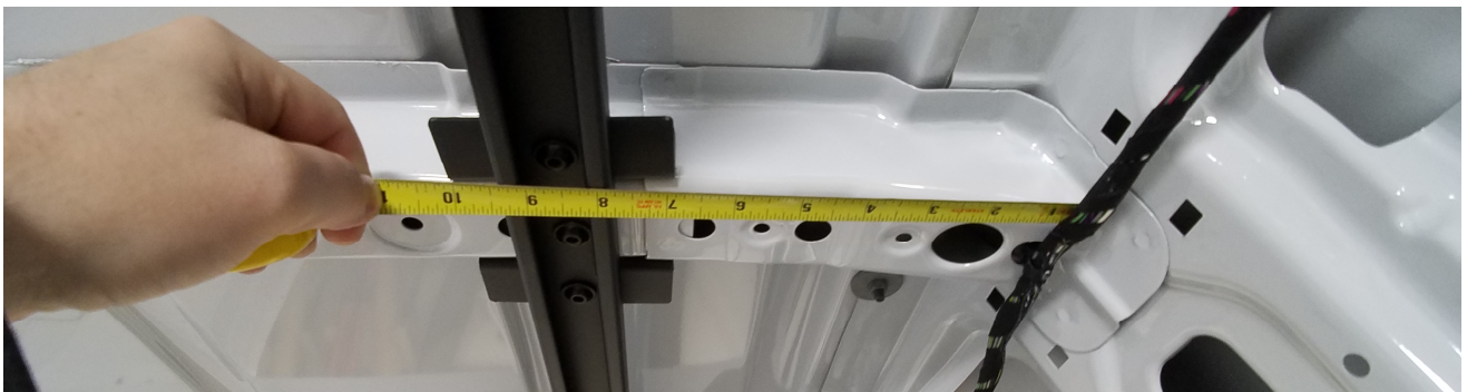
-All ceiling rail holes are factory holes to be widened, and are located in a line about 8.5" from the corner of the ceiling ribs.
