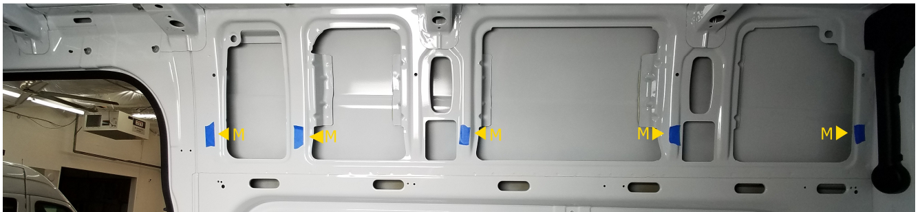
-Rear passenger hole locations (all manually drilled)
