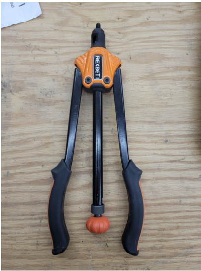
Required: Rivet Nut Installation Tool with 5/16 Mandrel
