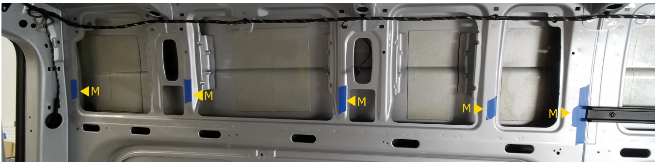
-Rear driver hole locations (all manually drilled).
