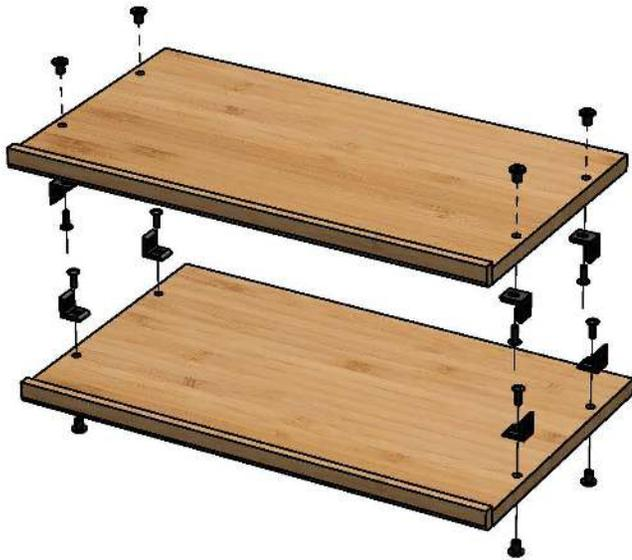
**3** Attach *small brackets* to shelf units using *hat nuts* and *small bolts*
