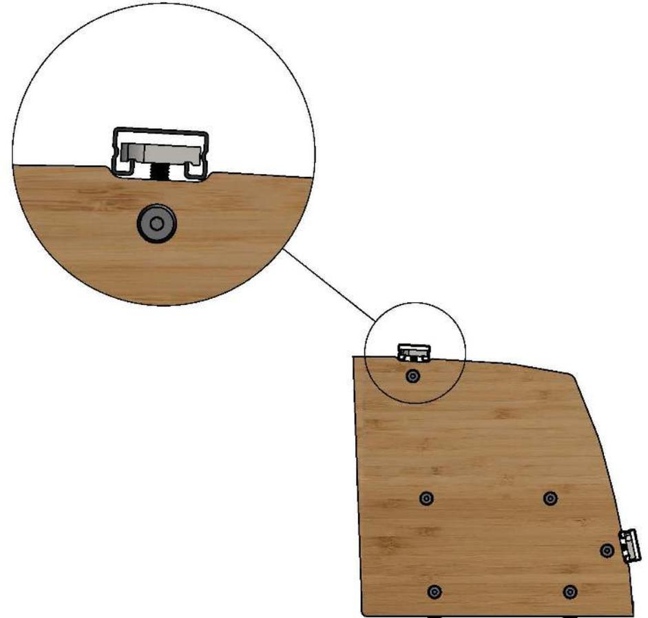
**1** Screw rail nuts to large rail bolts until nut is flush with top of bolt
