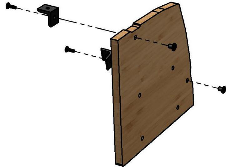
**2** Attach large brackets to end cap using hat nuts and small bolts. Attach end cap to mounting kit see, **APPENDIX P. 8**
