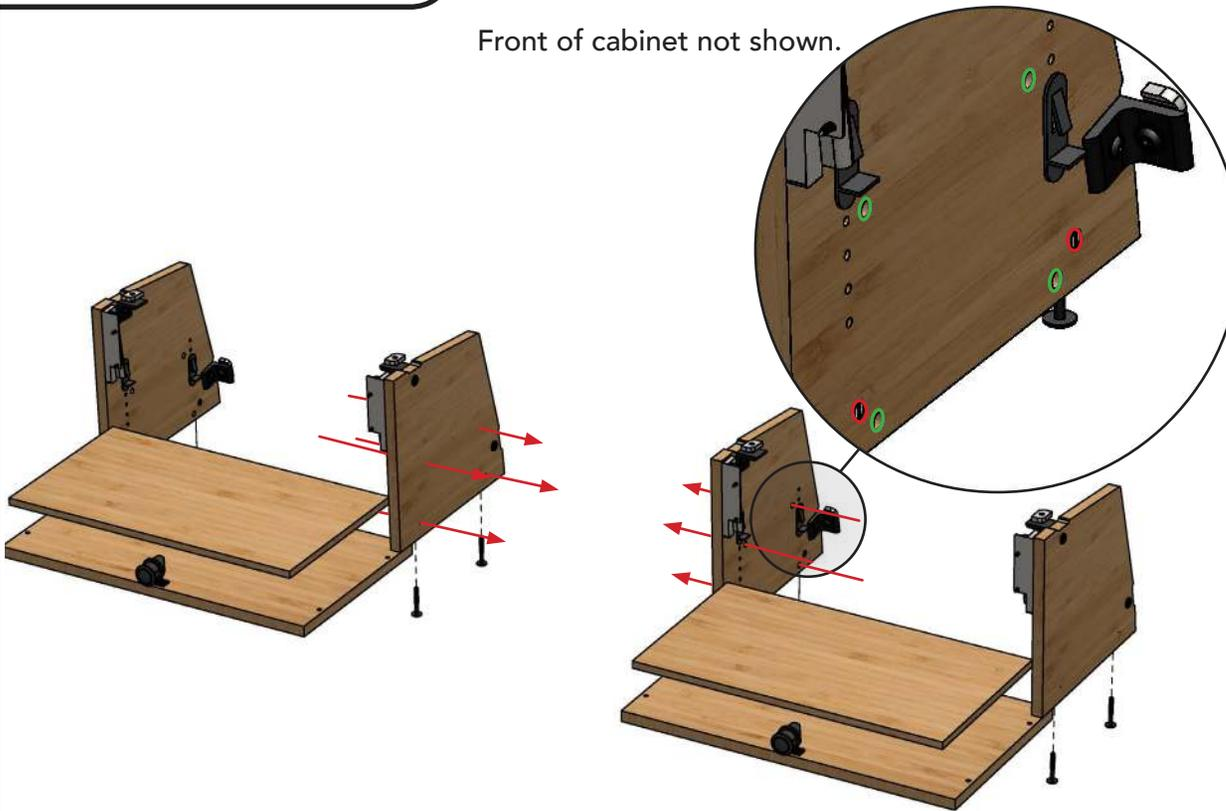
**1** Remove shelf and bottom from existing cabinet and drill through the 4 existing hole markers with a 3/8" drill bit, shown in green.
