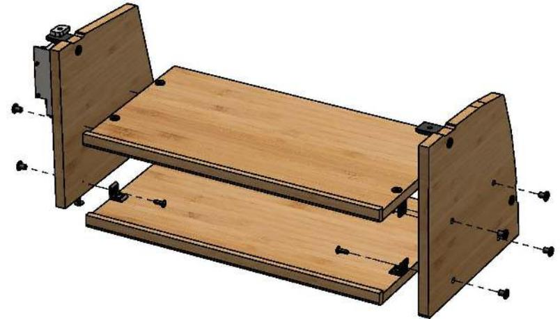
**4** Attach shelves to existing cabinet and end cap using *small brackets, hat nuts, and small bolts*.
