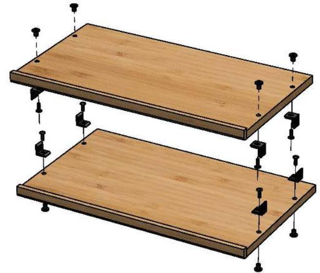
**2** Attach *small brackets* to shelf units using *hat nuts* and *small bolts*
