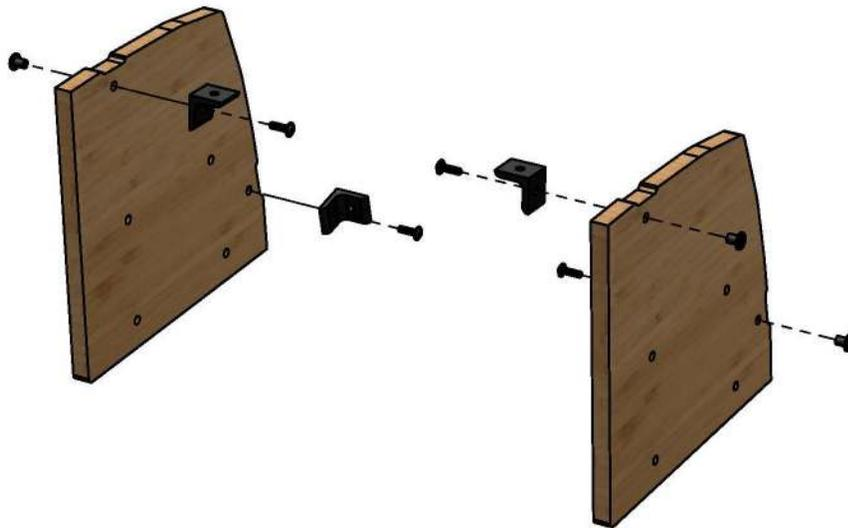
**1** Attach *large brackets* to shelf end caps using *hat nuts* and *small bolts*
