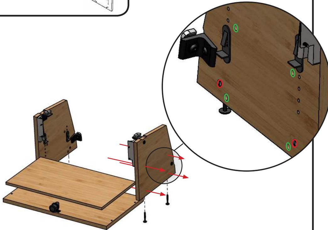
**1** Remove shelf and bottom from existing cabinet and drill through the 4 existing hole markers with a 3/8" drill bit, shown in green.
